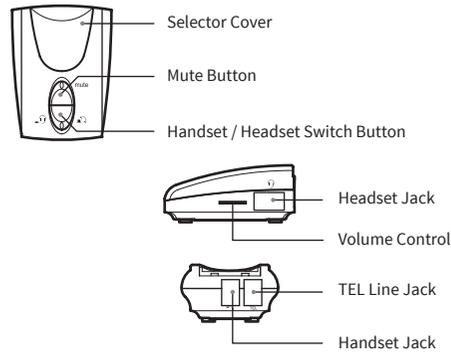
Once connected slide back the selector cover to reveal the setup switches which are unique to your individual telephone. Slide the top switch marked "1 2 3 4" to a position where you get clear sound and speech on a test call. The bottom switch marked "A B" is for the microphone type. Most headsets use the "A" setting but simply switch to "A or B" to turn on the headset microphone. Once you have reached the correct set up slide over the cover to conceal the switches.
