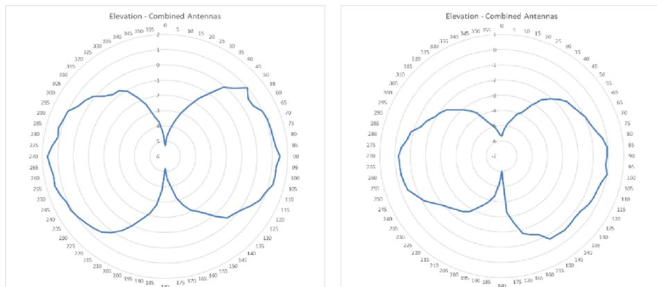
RG-AP730-L 2.4GHz (Left) and 5GHz (Right) Elevation Antenna Patterns
